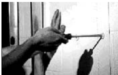
Frequent use of some hand tools can cause wrist problems such as carpal tunnel syndrome.
